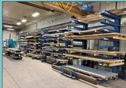
HD Cantilever Racks with Raw Sheet Stock
