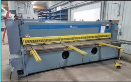
3/8" X 12" Niagara IF-12-3/8 Hydraulic Squaring Shear
