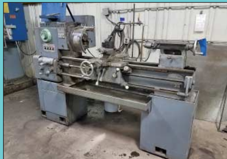
15" x 36" Cincinnati Hydra-Shift Lathe
